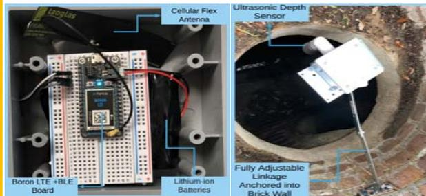
Figure 2. Installation of Sensor Nodes
